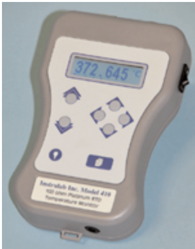
Shown with optional case and RTD sensor. For sensors, see 830/840 data sheets.
